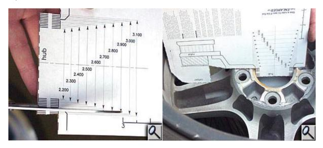
Once you have trimmed the hub area of the template, place the template into the back of the wheel. The hub area of the template should fit down into the hub hole in the wheel. This "Extreme" system template fits into this wheel with one exception; the template is resting on the spoke of the wheel and not allowing the template to rest flat on the hub section of the wheel. Also note that the template is very close to hitting at the top of the wheel to the top of the caliper.
