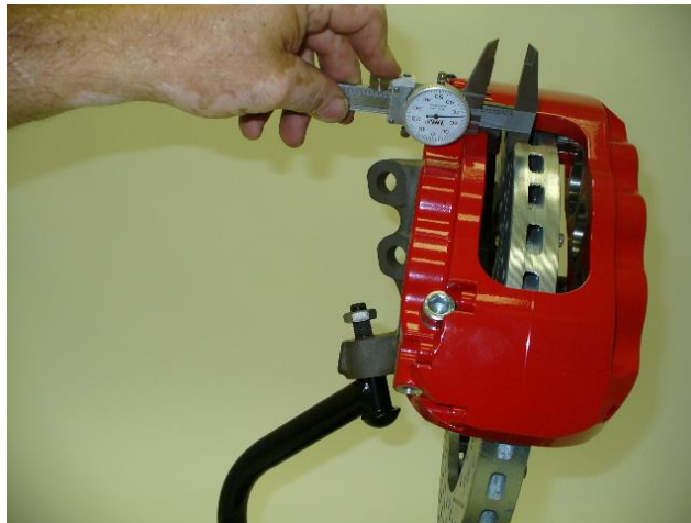
Measure gap from caliper body to rotor.
